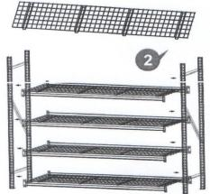
1. Pick up one Cross Beam (part B) and attached to the column of Upright Frame (part A) by inserting the two clips on the bracket of Cross Beam into the two keyholes of the column. You need to insert the clips starting from the outside and then tap down to seat the beam into the column in place.
